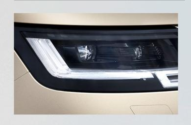
Digital LED headlights with industry leading microprocessor and 1.3 million micromirrors, can focus on 16 objects simultaneously and blank out reflections.
