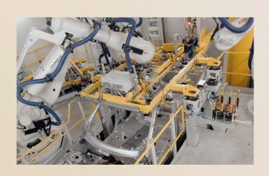
Smooth laser-welded interface rather than a traditional roof finisher provides a seamless finish in support of Land Rover's design philosophy.
